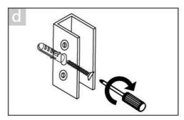
Fasten the wall brackets with ST4\*30 screws.
