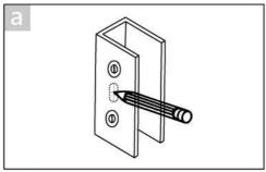
Position and level the wall brackets. Mark the fastening holes.
