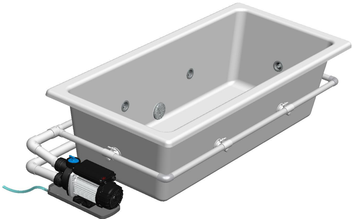
Figure 5 - Typical Indoor Installation with pump at one end
